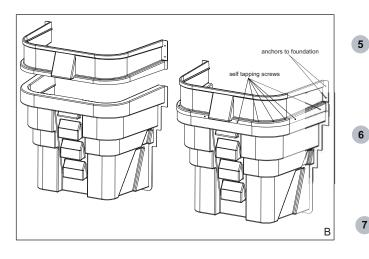
All Wellcraft wells are designed to Meet IRC 2003 International Residential Code 8 requirements, Section 310, for Emergency Escape/Rescue window opening for one and two family dwellings. The 2060 well is designed to be used with up to a 4 foot side sliding window that meets the egress code. 10-year limited warranty on window wells in effect when installation instructions are followed. Contact Wellcraft, Inc. for details,
